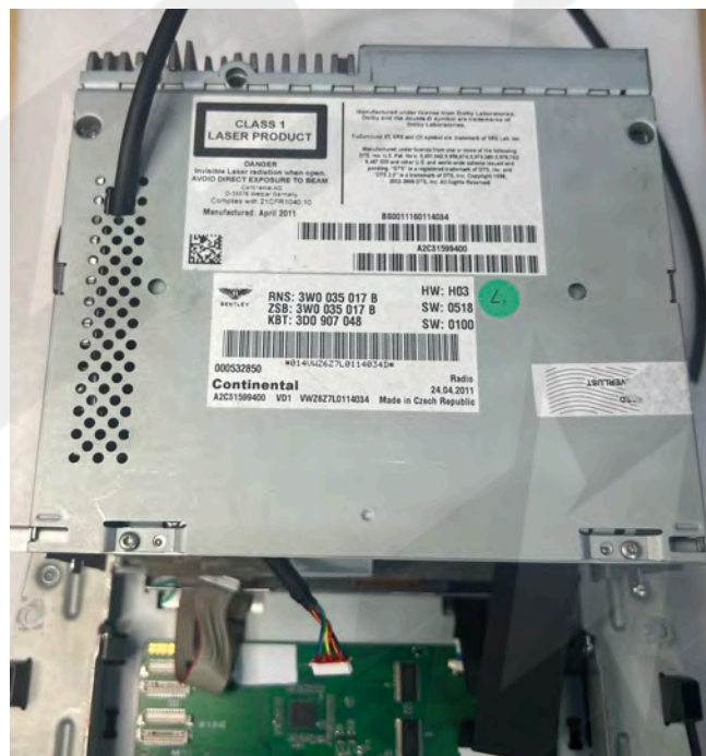
10. Run the provided PCB cable through the hole drilled in the top plate from step 5. Reconnect (2x) OE cables removed from step 3.
