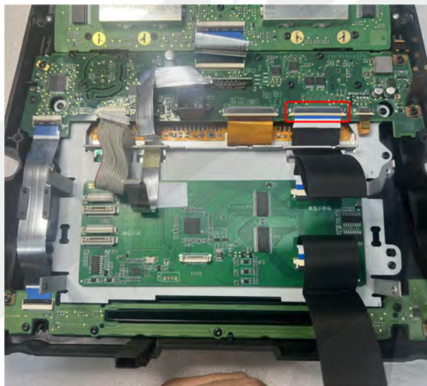
8. Place the provided PCB down using the double-stick to the back of the screen like shown. Connect the upper black ribbon from the PCB to the OE connector (removed from step 7) like shown.
