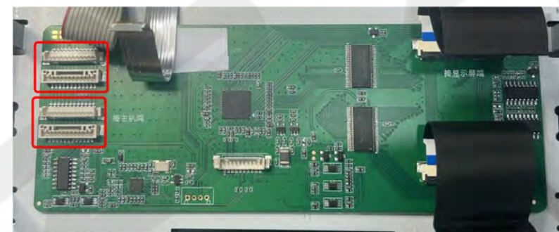
NOTE: these connectors are not used. Only the ribbons with black covering are used for this integration.
