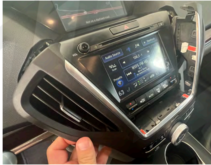
2. Pull the panel (including vents) forwards towards you - its held on with clips only.
