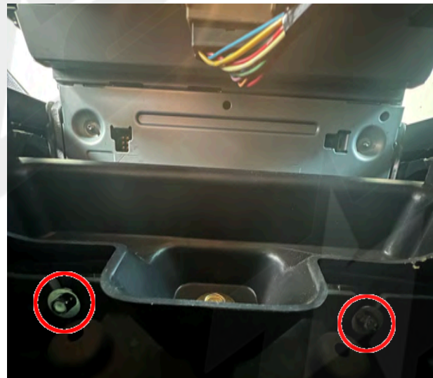
5. Remove (2x) 8mm bolts (firing upwards) underneath radio securing it to the sub-dash.
