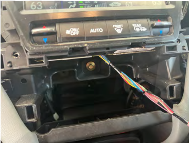
4. Remove harness connected to controller panel.
