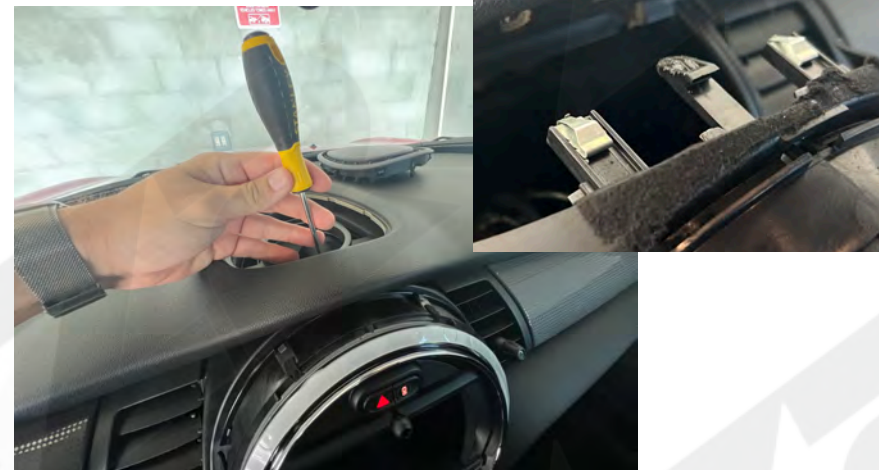
5. Locate center hole (circled), and using a Philips Head screwdriver (or similar), press the release tab downwards which secures the radio into the sub-dash. It takes a little effort to pull the radio outwards - it flips down from the top side.
