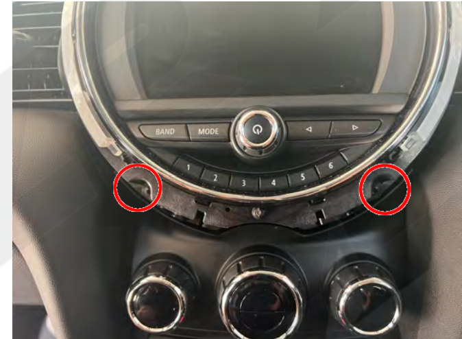
3. Remove (2x) Torx T20 screws.
