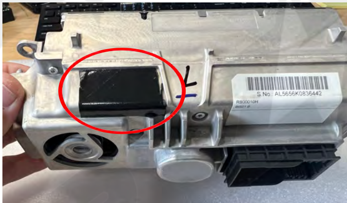
18. Using a piece of double-stick tape (not provided), secure the (2nd) sub-pcb to the radio securely. Clean the spot first to ensure it sticks.
