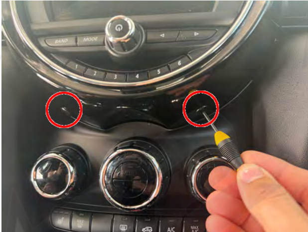
1. Using a straight pick (or similar), press in the center of (2x) release tabs (beneath radio surround) and remove.
