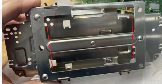
12. Using a saw or dremel tool, cut and discard the center support (only) to allow for the sub-board to be secured freely (future step).
