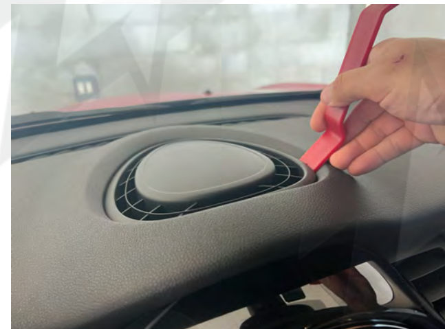
4. Using a plastic tool, pry and remove top vent.
