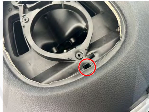
5. Locate center hole (circled), and using a Philips Head screwdriver (or similar), press the release tab downwards which secures the radio into the sub-dash. It takes a little effort to pull the radio outwards - it flips down from the top side.
