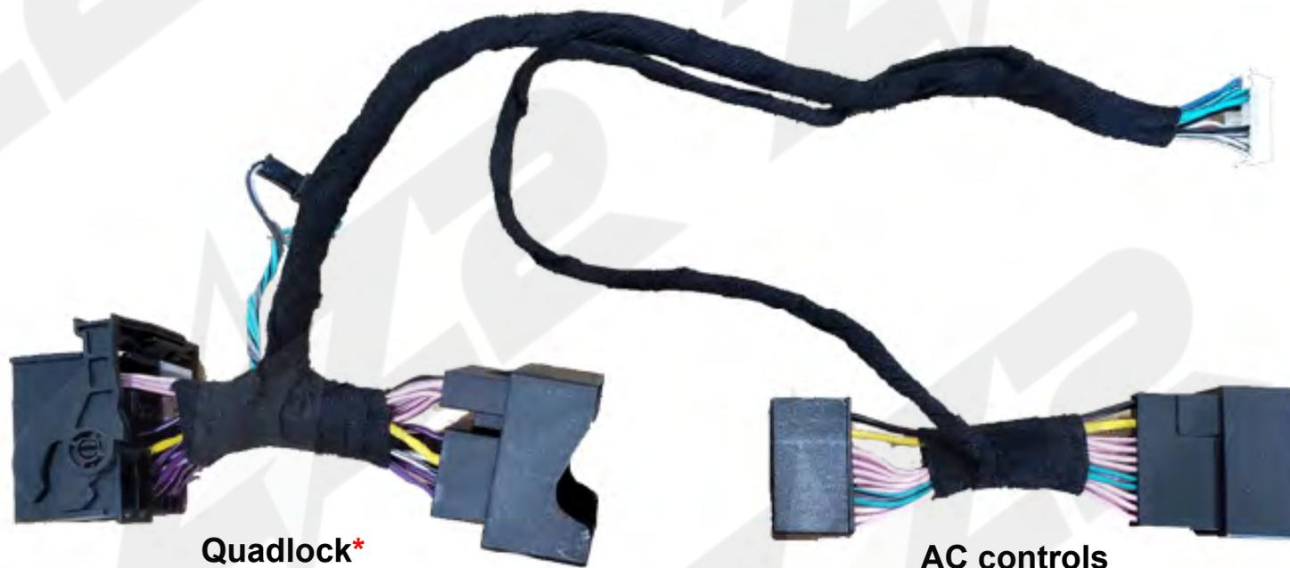
**\*If the car is equipped with fiber optic, please remove it from the original quadlock and move it to the supplied plug and play harness.**
