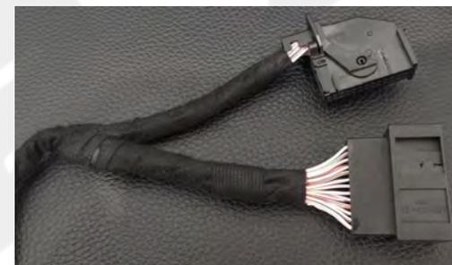
**For Q3-N (nav equipped), the secondary T-Harness (cam lock) is not used.**
