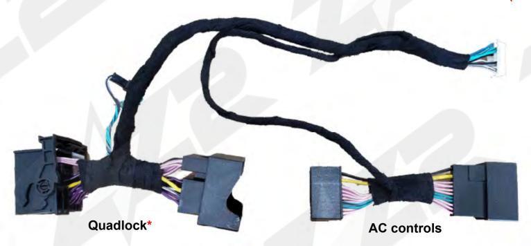
\*If the car is equipped with fiber optic, please remove it from the original quadlock and move it to the supplied plug and play harness.
