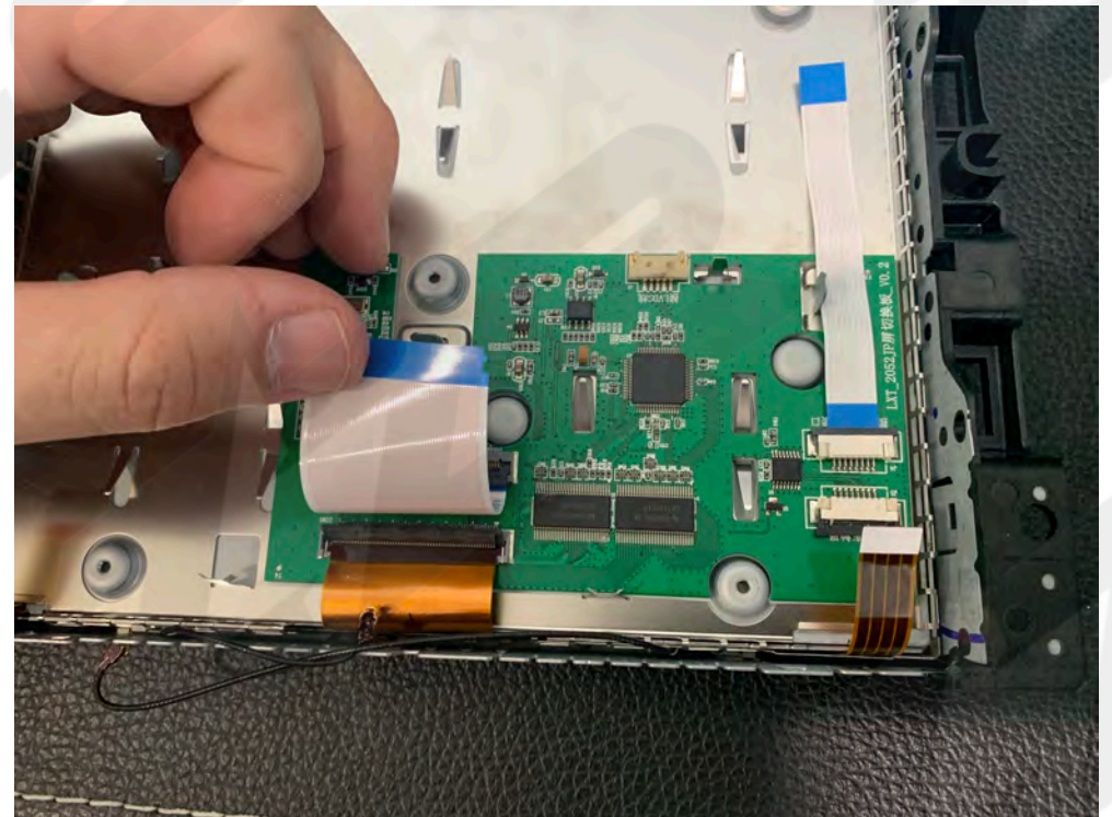
10. Place the provided PCB down (with protective backing) into place - all pegs and screw mounts should pass through and align the board properly.
