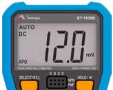
3. If the multimeter continues to show 0, disconnect the red lead from the tested wire and test another wire until the multimeter shows 12V.
