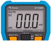
2. When ACC is OFF, the multimeter shows 0. Turn the motorcycle key and observe the multimeter. If the tested wire is ACC, the multimeter should show a voltage of 12V.
