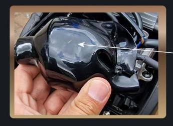
When closing up the waterproof sock please ensure that the connectors are fully covered prior to tightening it up with a cable tie.
