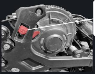
Loosen the highlited bolt to allow the tension lever to be removed. This will allow you to remove the motor pulley cover.
