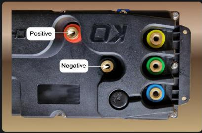
When you reconnect your controller it is very important to note that all of the connectors are colour coded. Please ensure that cables are fitted to the corresponding correct colour to prevent malfunction or damage to the unit.
