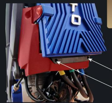
When fitting the controller we would recommend starting with the top and working your way downwards. Please note that the controller mounts over the plastic protector at the bottom.
