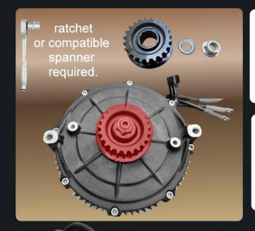
The pulley can be removed using an appropriate ratchet or spanner. This can be a little tricky as the bolt is normally very tight. We would recommend clamping the pulley with rubber grips to allow sufficient force to be used without damaging it.
