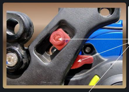
Ensuring you have the right tension on your belt is very important. To do this you need to loosen the bolt highlighted and slide the motor up and down engaging the lever until the correct tension is achieved.
