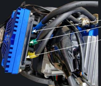
Prior to fitting the plastic cover between the bashguard and the controller ensure your waterproof sock and all cabling are tidy and free from snags (use cable ties where appropriate).
