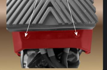
Remove the indicated bolts and screws to release the plastic cover and give access to the bottom of the controller.
