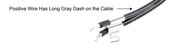
The positive wire (with long gray dashes) gets wired to positive power in the vehicle and the negative wire gets wired to common or ground in the vehicle. If you experience "engine noise" when you press the gas pedal you may need to move to a better ground source.
