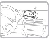
B. Orient the adhesive foot so that Edge is easily accessible. Loosen the knob and adjust the adhesive foot to position 1 or 2, and then tighten it.
