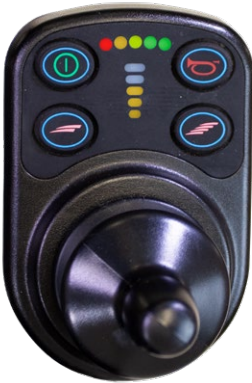
BATTERY CHARGE INDICATOR ON JOYSTICK CONTROLLER
