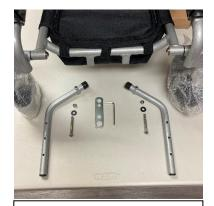
With the old footrest removed. Place both adjustable legs with the drilled holes facing out
