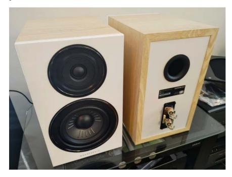
This Klarity woofer is mated to a new 1" woven polyester dome tweeter, which is pretty much par for the course for this type of speaker. According to Wharfedale, the tweeter's flat front plate and magnet system allow for wide dispersion, providing a wide sweet spot and filling the room with sound.
