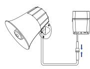
2. If using an external 12V DC power supply, connect the cable to the controller at this time. With the power source off or unplugged, connect the cable of the 12V DC power adapter or power supply to the 12V DC input of the alarm controller.
