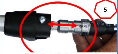
Be sure to Align Snap Lock Holder's drilled hole with Snap Lock Set Screw. Then begin to insert Snap Lock into the Snap Lock Holder.
