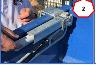
Remove & Discard broken Pivot Arm Tube & keep Button Head Bolts. 2 extras (if needed) are in shipment.
