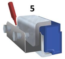
Apply Red Threadlocker to about 3 threads on each bolt behind the Compression Bracket.
