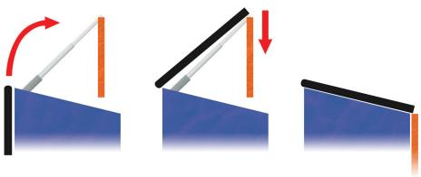
After installation, lift arm up using guide below, place lid onto the arm and close using Nylon Strap, like shown below.
