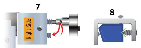
Continue fasting the Cone Point Bolts with the 1/4" Hex Drive, being sure to alternate between each bolt to ensure even pressure and alignment. Tighten until Cone Point Bolts are firmly pressed in the side of the Dumpster.
