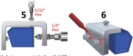
Lightly fasten cone point bolts with 1/4"
