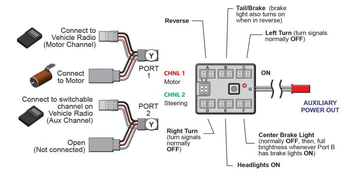
Note: 1. Hazard Lights (All LEDs turn off except ports B & D that blink as hazard lights after 20 sec). You can turn OFF Hazard Lights by press-and-hold the Mode Button for 3 seconds. Repeat to turn back ON.
