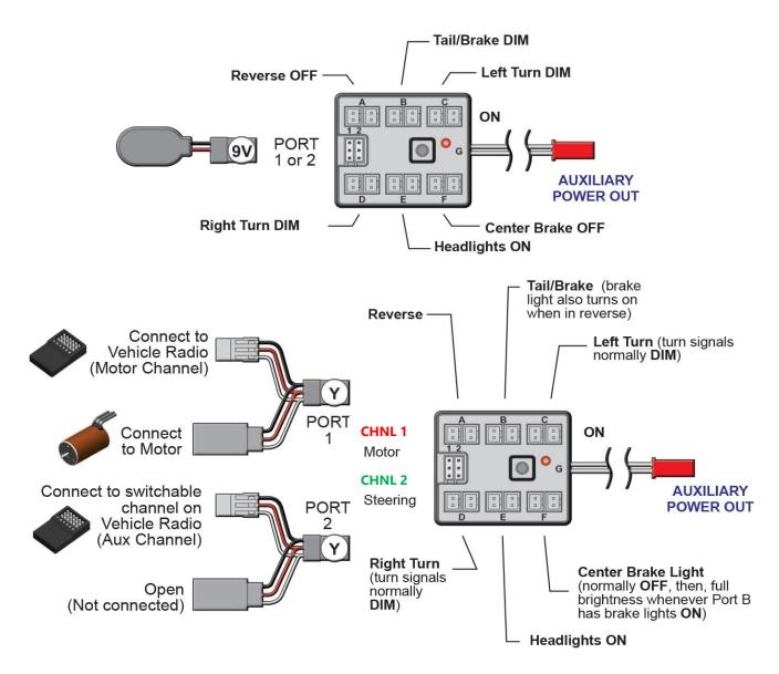
Note: 1. Hazard Lights (All LEDs turn off except ports B & D that blink as hazard lights after 20 sec). You can turn OFF Hazard Lights by press-and-hold the Mode Button for 3 seconds. Repeat to turn back ON.
