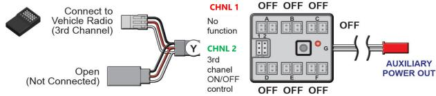
Note: ON/OFF function on 3rd Channel (including Pig Tail)
