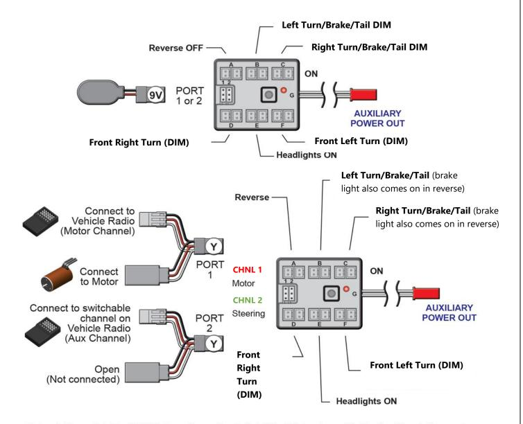
Note: 1. Hazard Lights (All LEDs turn off except ports B & D that blink as hazard lights after 20 sec). You can turn OFF Hazard Lights by press-and-hold the Mode Button for 3 seconds. Repeat to turn back ON.
