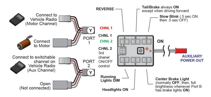
Note: 1. Hazard Lights (All LEDs turn off except ports B & D that blink as hazard lights after 20 sec). You can turn OFF Hazard Lights by press-and-hold the Mode Button for 3 seconds. Repeat to turn back ON.
