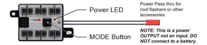
The UF-7R has many different pre-programmed output MODES to fit multiple lighting requirements. Pressing the MODE button scrolls through the various modes. 0-10 and back to 0.
