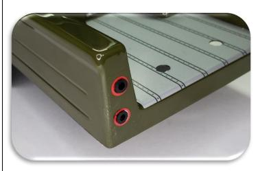
4. Snap LED holders into the body from the outside. Insert LEDs into LED holders from the inside of the body.
