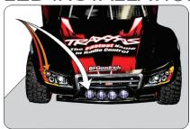
1 Choose where to install, what size, and what color LEDs are to be used. Next, choose the desired UF7B blink MODE (See Blink Mode Section page 5).
