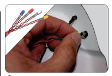
4. Insert LEDs into LED Holders. It is recommended to apply a pliable glue, such as Zap Goo or Shoe Goo, liberally making sure the glue contacts the body, the LED and LED wires. The glue should strengthen the wires and help the LEDs last longer.
