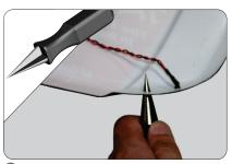
2. Drill Holes for LED Holders. Be careful to not drill the hole too large.
