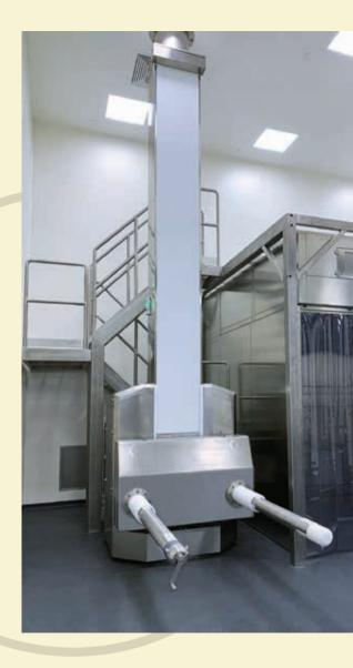
The VCS transports the powder in an air flow and is vacuum sucked through stainless steel and polyurethane pipes, without electrical parts.
