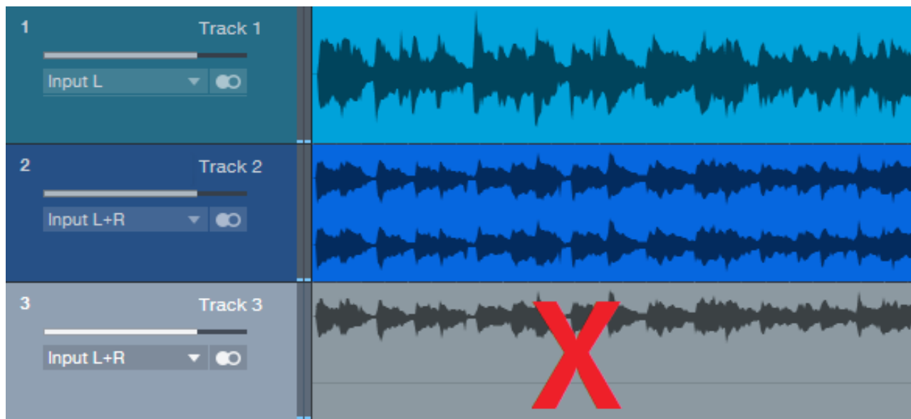
Figure 1: With Helix Native, it's best not to record the guitar into one channel of a stereo pair. However, the track output should always be Stereo.
