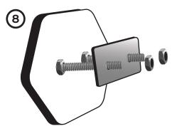
Place the 2 provided nuts from your insert onto each of your rods, tensioning evenly.
