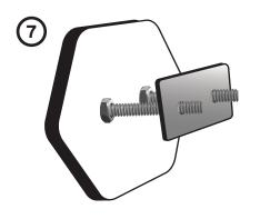
Take back plate and insert into 2 rods while holding grill badge from front side.
