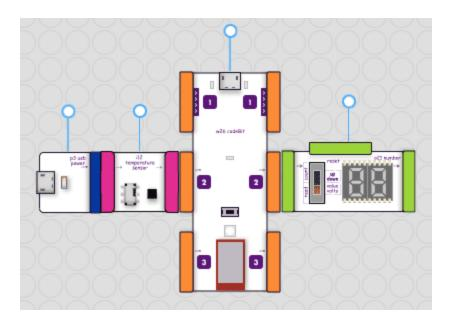
To start building a circuit, just click and hold on a Bit and drag it onto the canvas. You can drag the colored edges of the Bits together to create your circuit.
