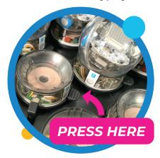
Located at the base of each charging cradle inside the Power Pack is a thumb tab. Gently press down on the tab to release the charging cradle.
