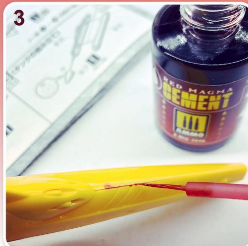
**2, 3.** Thanks to the brush built into the lid, the glue can be applied with the joint with precision, allowing it to flow through by capillary action.
