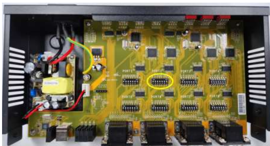
Figure 3.10 - ES-U-3008-RMC has a set of 7-way DIP switches for each port (one set circled)
