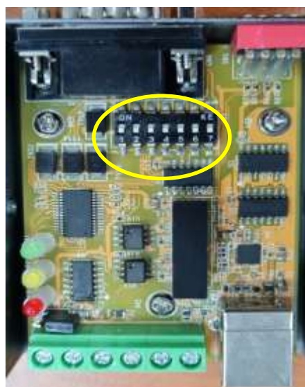
Figure 3.10 - ES-U-3008-RMC has a set of 7-way DIP switches for each port (one set circled)
