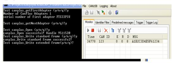
Then you can monitor the standard CAN frame transmitted on CAN network.
