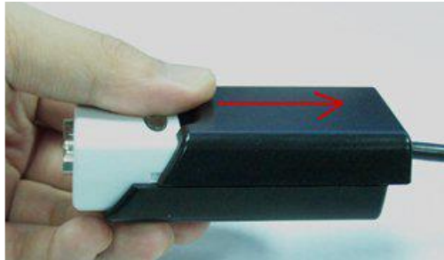
Figure 1 – Push down the upper case and slide it to open
