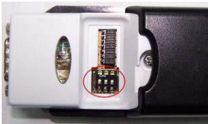
Figure 2 - 3-way DIP Switch for Operating Mode Selection
