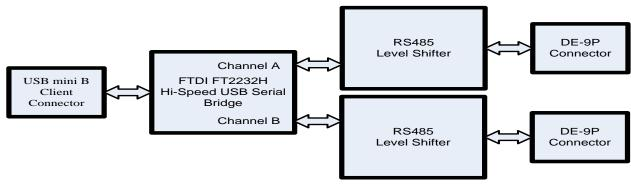
Figure 1.2 USB2-H-5002 Block Diagram
