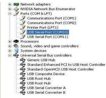
Figure 2.10 - COM Port Assignment
