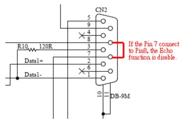
Figure 2.3 USB2-H-5002 Termination resistor and echo disable
