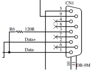
Figure 2.3 USB-COM485-PLUS1 Termination resistor
