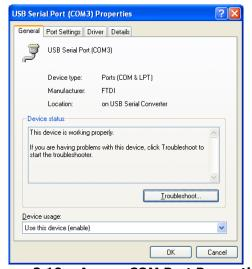
Figure 2.10 - Access COM Port Properties
