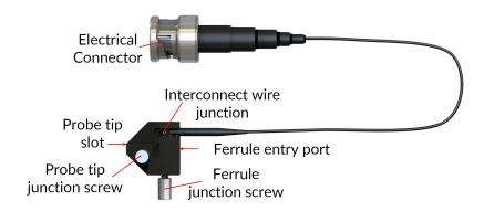
Figure 2.2: Single-cell Opto-electric Probe Adapter
