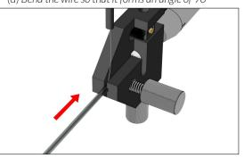
(f) Push the probe to create a contact with the zirconia ferrule
