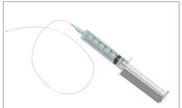
(c) Block the plunger with a syringe stopper to keep the hollow-core under negative pressure
