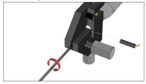
(g) Rotate the probe in the receptacle to align the two optical cores
