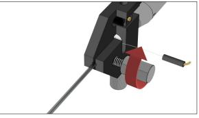
(h) Secure the probe tip position using the probe tip junction screw
