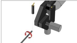
(e) Align the interconnect wire with the slot
