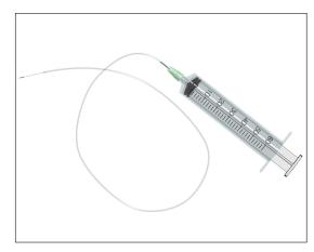
(a) Put a plastic tube at the tip of a large volume syringe and install the probe tip at the end
