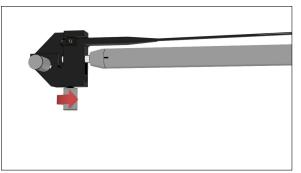
(a) Insert the opto-electric probe holder in the adapter
