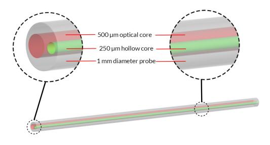
Figure 2.5: Single-cell Opto-electric Probe-Raw Fiber
