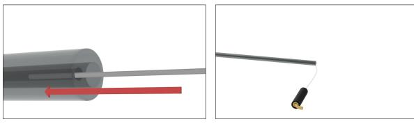
(c) Insert the wire inside the hollow core
