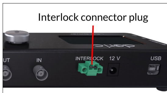
(a) Interlock connector plug connected
