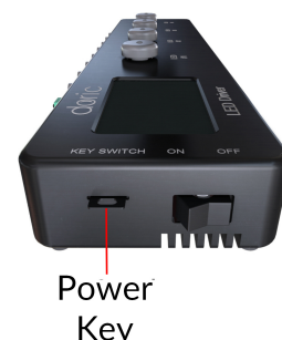
(b) Properly inserted key switch
