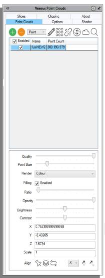
When a point cloud is added and selected in the displayed list, a number of options become available which control the appearance of that point cloud. **Note:point cloud must be selected for the following features to work:**
