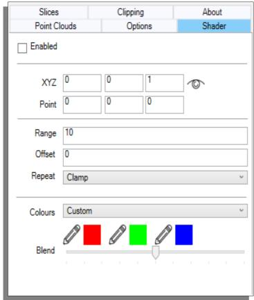
The shader panel provides control over the planar shader. This is a capability which colours data along a plane or vector from a given position or offset.
