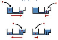
Asymmetrical volume loading of chambers is particularly useful when it is desirable to fluidically isolate a chamber from its adjoined partner. Since the flow across the microchannels will be towards the chamber with the relatively lower fluid level, the chamber with higher relative fluid level <u>will not be</u> exposed to molecules that have been specifically added to the chamber with the lower level of fluid. Importantly, the chamber with the lower fluid level <u>will be</u> exposed
