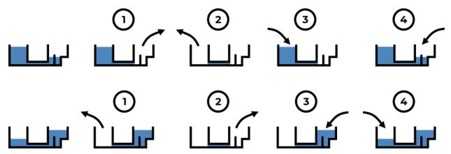
In addition to chamber isolation purposes, asymmetrical volume loading of chambers is useful when it is desirable to induce a flow through the microchannels. For example, this might be the case when coating the microchannel surfaces or chemically fixing neuronal projections located within the microchannels. Also, asymmetrical volume loading is necessary to allow antibody access to epitopes located within the microchannels when performing immunohistochemical staining procedures.
