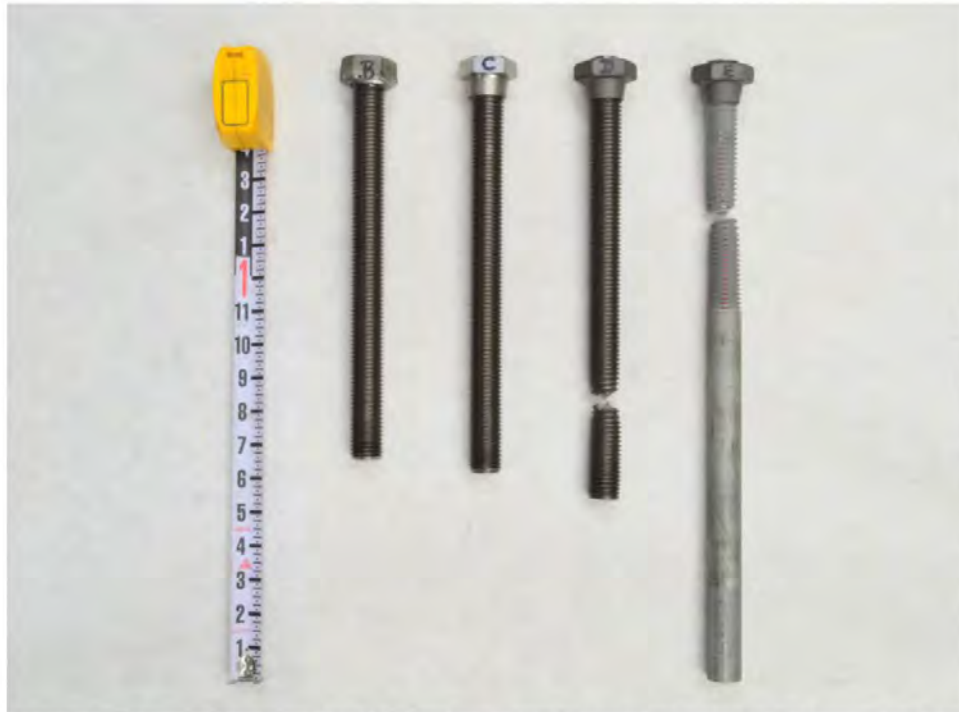
(a) Rod-nut assemblies after testing - assemblies B, C, D and E from left to right
