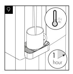
The temperature of cold water can be set from 4c to 11c.
