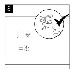
When the cold water switch is turned on, the cold water and indicator will be lit.
