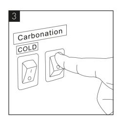
After completing the water installation, turn on the sparkling power switch and the pump will run. Do not open the regulator valve until the carbonated switch has been turned on.
