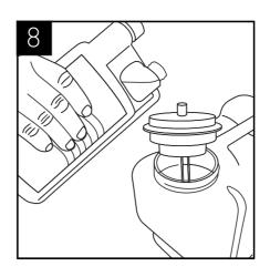
If a Waste Overflow System is fitted, empty this and flush through with a small amount of sanitisation fluid if needed.
