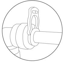
**IMPORTANT!** ALWAYS ENSURE SECURITY CLIPS ARE USED ON ALL WATER AND CO2 CONNECTIONS.
