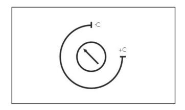
This shows the correct and factory default set point. Although adjustment is possible (clockwise reduces the temperature and anti-clockwise increases the
