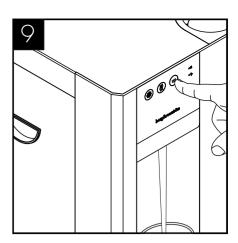
When the external cleaning (after a minimum of 5 minutes) is completed, flush the machine using the chilled button with clean water until the dispense water runs clear. Repeat briefly with the ambient button.
