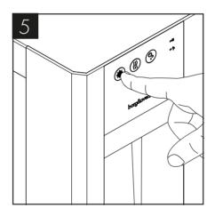
All hot & sparkling tanks must be purged of air by holding the corresponding button. Do not switch the hot system on until tank has been purged.
