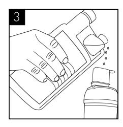
Add 25 ml of Sterizen® 30 Internal Water Cooler Sanitiser fluid to a clean and empty service filter cartridge.
