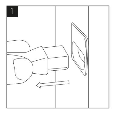
Please make sure the machine is completely disconnected from the electricity before carrying out any maintenance work.
