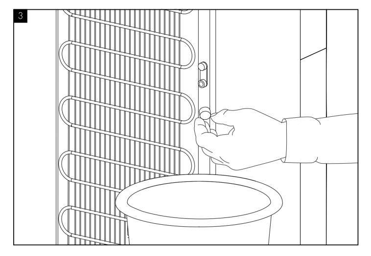
To drain cold and ambient units, simply push each dispense button until no water dispense. For cold and hot dispensers push the dispense until no water dispenses and then remove both drain port caps to empty the water tanks.
