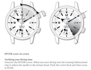
You can read off your diving time from the minute hand on the graduations of the rotating bidirectional ring. The example shows: 15 minutes diving time.
