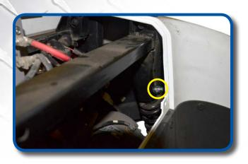
Remove upper bolt from rear shocks on both sides. Retain hardware.
