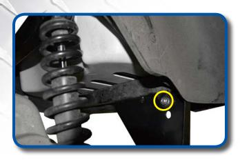
Attach sway bar bracket using hardware provided.
