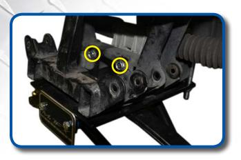
Attach front of Main Suspension Assembly to frame as shown using provided hardware.
