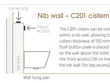
The C201 cistern can be installed within a nib wall, allowing for a cistern thickness of 130 mm. The flush button plate is placed either on the wall above the toilet pan (for front access) OR on the top of the nib wall (for top access).
