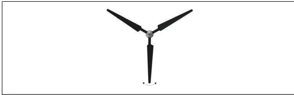
Fig. 7: Balancing the rotor (Y position)
