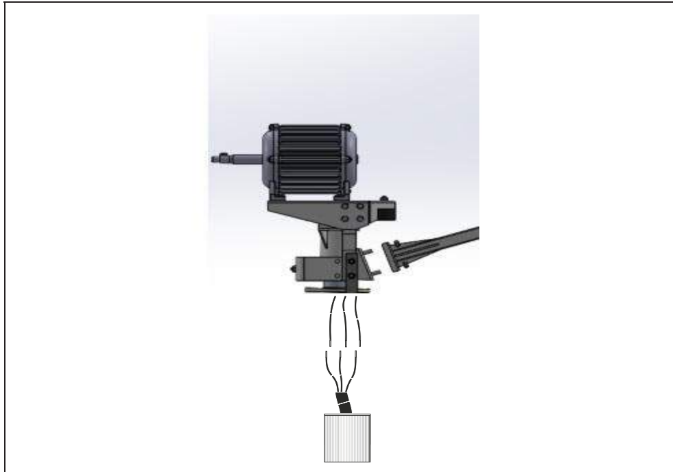
Fig. 8: Connecting the three-wire cable to the generator
