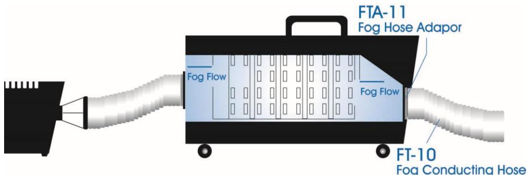
During operation, if you experience mechanical noise or no output, unplug immediately. Check power connections and fog machine operation. Wait three minutes and then plug the unit in again. After plugging the unit in and turning it on, wait for two minutes. If the problem persists, discontinue operation and return the machine to your ANTARI dealer.
