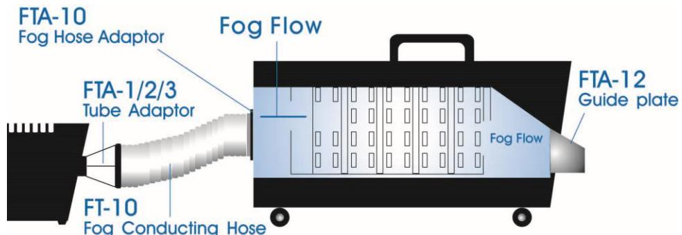
In the second example, substitute the guide plate (FTA-12) with a fog conducting hose (FT-10) that attaches to the front of the fog cooler via an adapter (FTA-11). This configuration allows the fog cooler's output to be guided to a desired area without being affected by air currents generated by movement, wind, fans or air conditioners.
