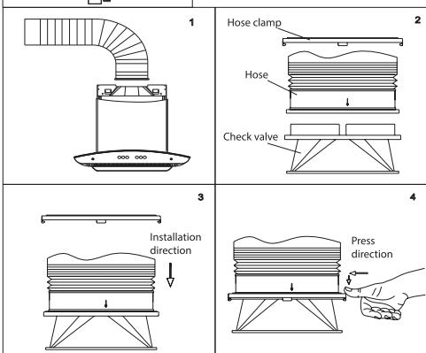
Install the pipe according to the picture.
