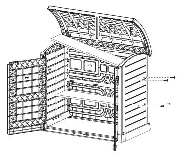
Shelves and screws are not included in the packing. Mark the locations of the screws to align each shelf, and screw tightly in position.
