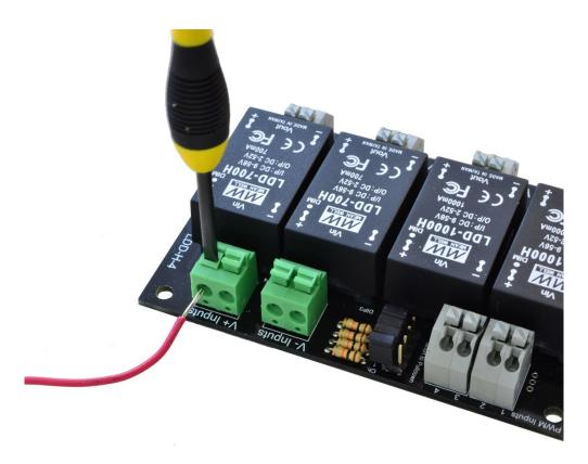
Repeat this process with the wire attached to the –V screw terminal on the SE-350-48, but insert it into the spring terminal labeled "V- Inputs."
