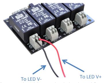
Repeat this process for all remaining channels being used on the board. From left to right with the board facing up, the channels are 1 through 4 respectively. In this picture, we are using Ch.1 on the board with a string of Solderless LEDs:
