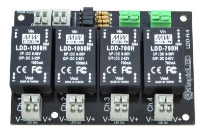
The LDD-H-4 board is designed to hold the LDD drivers firmly and the drivers are not meant to be removed once they are installed. We do not recommend removing the LDD drivers from the LDD-H-4 board. Removal can result in damage to the driver and will void any warranty.
