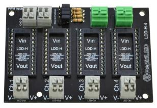
Align the pins on the driver with the driver sockets and press the driver down firmly until it is fully seated in the socket. It's best to do this with your thumb in the middle of the driver. Make sure that the pins are aligned before pressing down so that the pins don't get bent. This is what the driver will look like on the board before and after installation:
