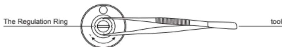
**Adjustment of thread connector:** The adjustable thread connector makes Lemo better matched with your battery. Just use the tool to rotate the word cross as needed.
